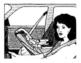
Your child may travel on the front passenger's seat only if you have a child restraint system which is specifically designed and approved by the child restraint system manufacturer for use in the front together with the restraint system installed at that position.
